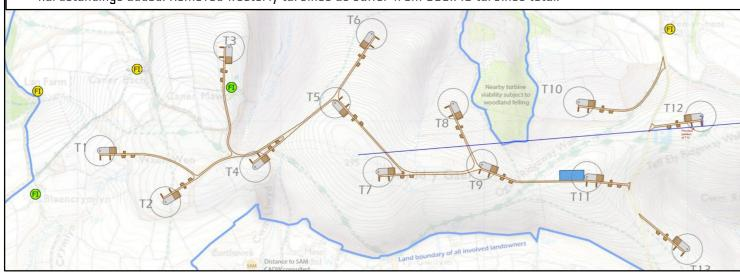
4 ) 2024: Candidate turbine VI62 198m tip. Telecoms operators confirmed areas suitable for turbines. Access route confirmed. Ecology study completed: turbine layout adjusted to avoid sensitive biodiversity. Water run-off areas identified and avoided to mitigate effects on lower properties. 11 turbines total, north-eastern turbine removed as buffer to Taff Ely.
